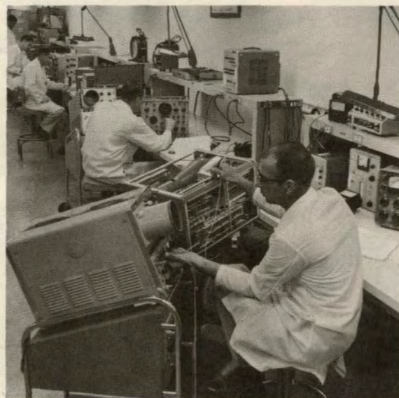
Periodic checks of line test equipment at MacDill AFB PMEL assures F-4 performance. A1C Robert Meyers, 47 TFS, calibrates Phantom's weapons control system with a Radar Test Set which, if misaligned by only .03 of a volt, can cause the F-4 system to be ineffective.
